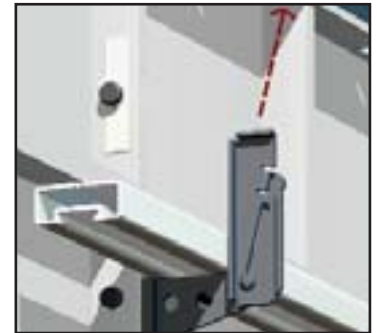
~Removal of waler board~
